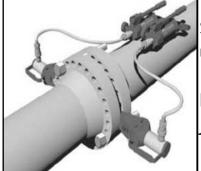
Strongly recommended that two K-SW15TE wedges be used on the flange joint positioned 180 degrees apart.
