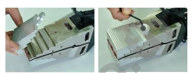
**ATTENTION!** When using the stepped blocks, ensure there is a minimum hold of 15mm (0.59") and that the full width of the block is used.
