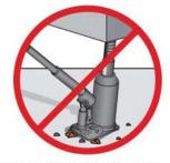
Every jack or ram, whether used individually or in a system, should be completely supported on a solid, firm, non-sliding foundation capable of supporting the load.
