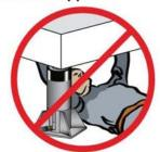
Hydraulic rams are not meant to be used as permanent supports, but are designed to lift and lower. If you need to hold the load for any length of time, cribbing or Powerram locknut cylinders should be used.
