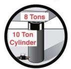
You must know the weight of what you intend to lift and choose a ram with at least 20% more capacity. Be aware of possible load shift requiring more capacity at the particular lifting point.
