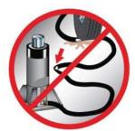
Do not drop sharp or heavy objects on hose. Keep hose out of heavy traffic areas. This will cause internal damage to hose wire strands. Applying pressure to a damaged hose may cause it to rupture. Avoid sharp bends and kinks when routing hydraulic hoses.
