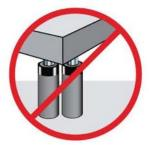
For multiple rams lift, you must be able to determine the location and number of lifting points that will allow the load to be evenly distributed to all the rams. This is called load balance. Size, center of gravity, and load geometry must be considered in order to correctly determine load balance.
