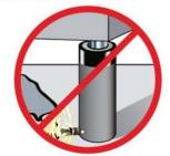
Never attempt to disconnect hydraulic hoses, fittings or couplers under pressure. Unload the ram, open the release screw on the hand pump and shift or open all hydraulic controls several times. If system includes a gauge, double check the gauge to insure pressure has been completely released.
